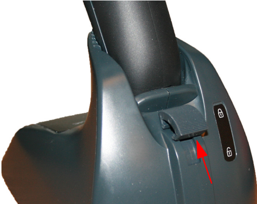
Figure 2. Lever in locked position
