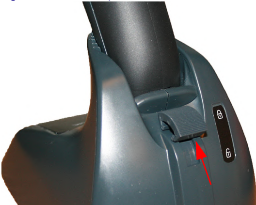
Figure 2. Lever in locked position
