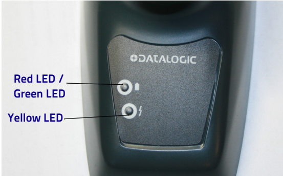
Figure 6. QuickScan Base LEDs
