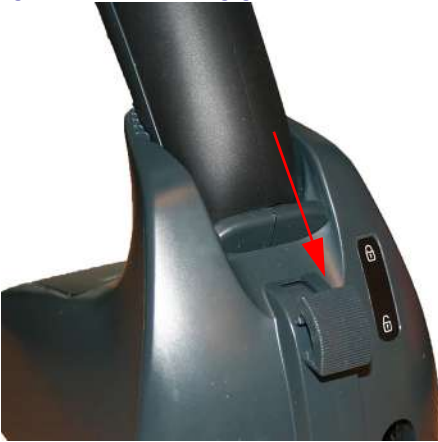
Figure 1. Lock lever disengaged
