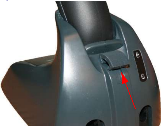
Figure 2. Lever in locked position
