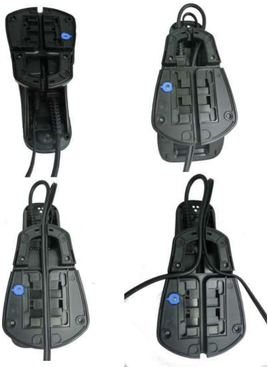
Figure 6. Options for routing the DC cord
