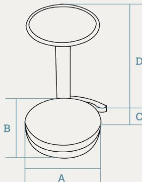
Dimensions of the plate:  $\varnothing$  232 mm.
